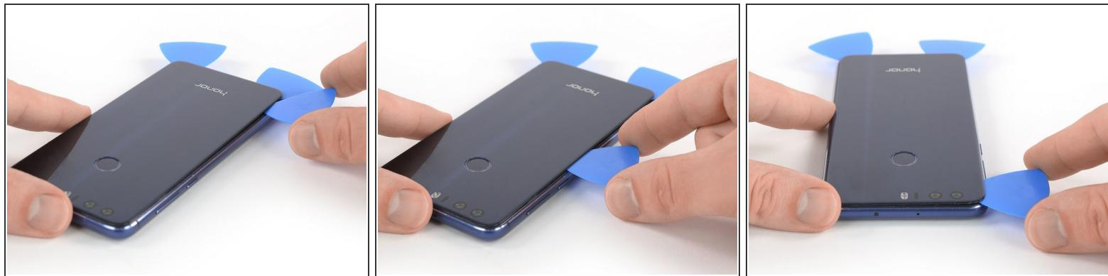
**⚠** The fingerprint cable is located above the power and volume buttons on this side of the phone. Only use the tip of the opening pick in this area to avoid damage.
