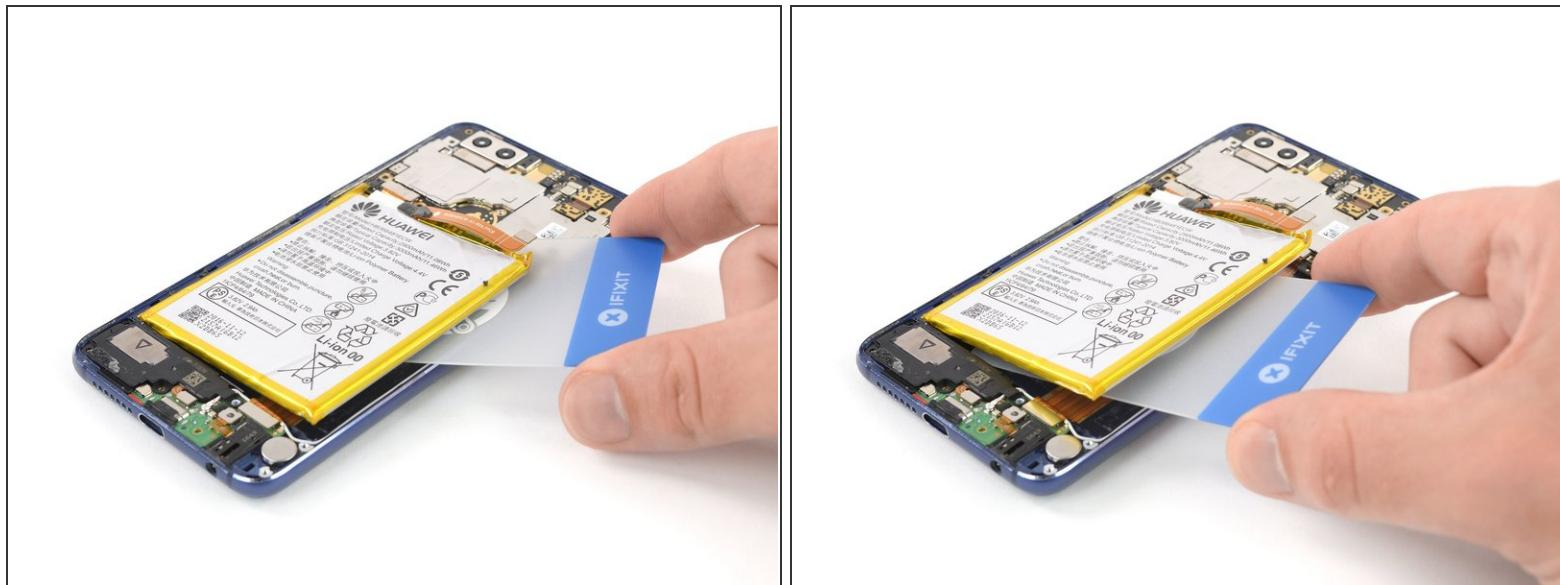
**⚠** The display flex cable and interconnect flex cable run underneath the battery. Be careful not to damage them while cutting the remaining adhesive.
